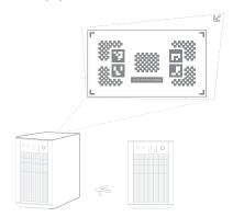
When the automatic obstacle avoidance function is enabled, the frame will automatically avoid obstacles if there are obstacles in the projection area.
